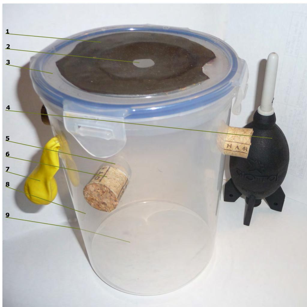
**Fig.4:** Ectoparasite collection device (ECD v6.2); 1) Flexible Thera-Band®, 2) Hole, to allow the bird free breathing, without inhaling chloroform gases; 3) Lit, with a perch fitted inside, to allow the bird to rest comfortably; 4) Jessops® Rocketblower; 5) 22 mm hole for gas circulation; 6) Wine cork; 7) Overpressure absorber; 8) Cylindrical Tupperware® container; 9) Whatman® 110 mm filter paper.
